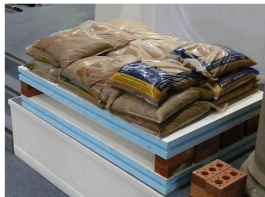
Long term testing of floor panel
