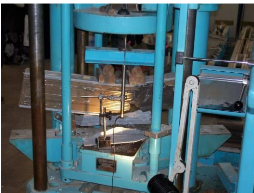
Testing ground beam to failure at Coventry University
