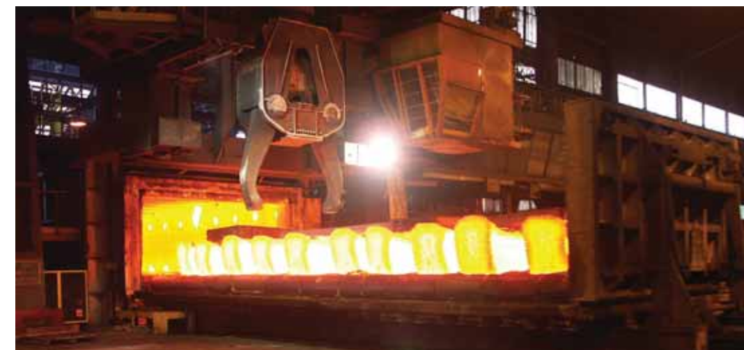
Left: Ingots being heated prior to rolling of Boat 4 NQ 1 Steel at Industeel
